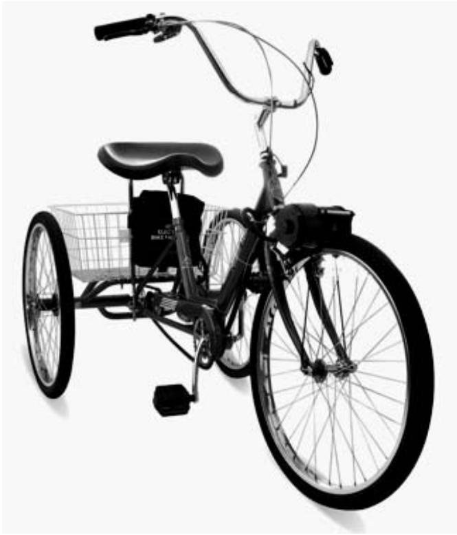
**Figure 18.** The Electric Bike Kit incorporated onto a tricycle.
