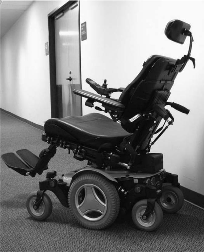
**Figure 2.** An electric power wheelchair.
