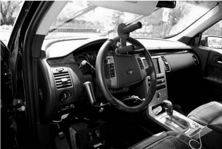
**Figure 2.** Hand controls for braking and accelerating.
