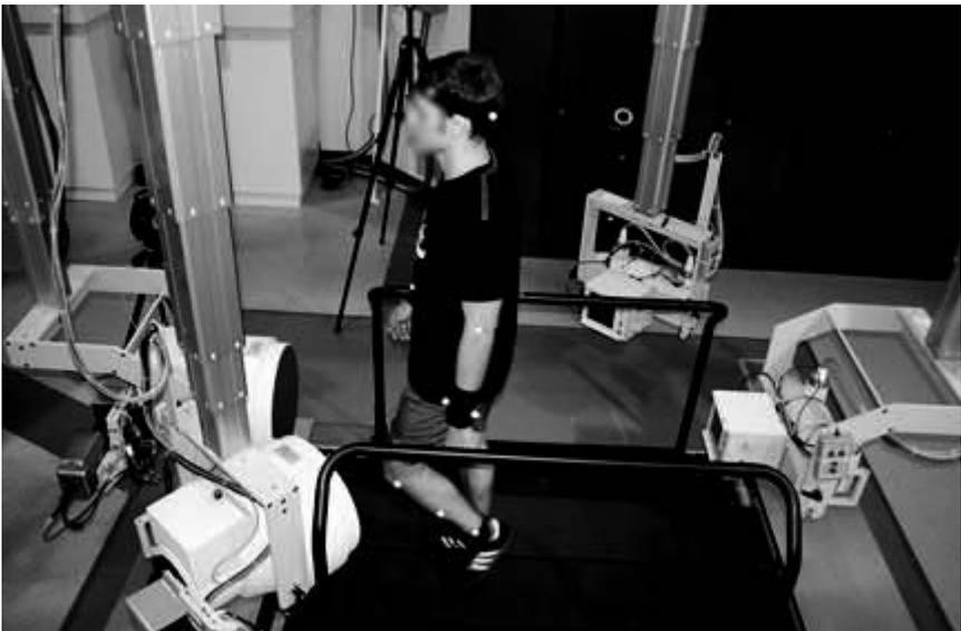
**Figure 4.** Biplane system for knee analysis (Image courtesy of Scott Tashman, Ph.D., Director of the Biodynamics Laboratory, University of Pittsburgh Department of Orthopaedic Surgery).
