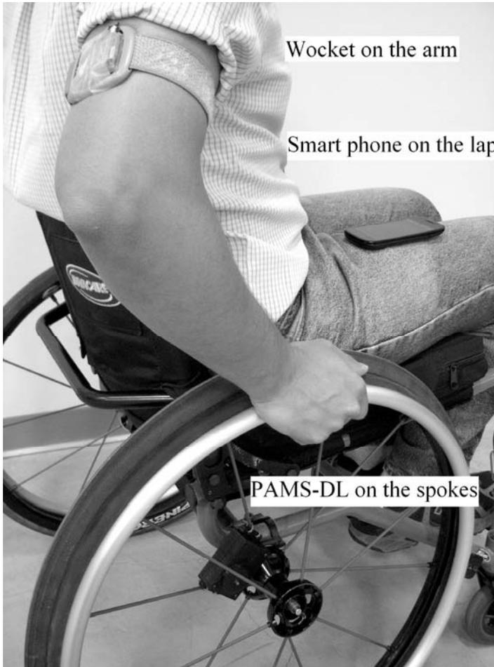
**Figure 6.** Investigator using the Physical Activity Monitoring System (PAMS). PAMS consists of a wheel rotation datalogger and a wearable accelerometer to detect wheelchair user's physical activity levels and provide real-time feedback via smart phone.
