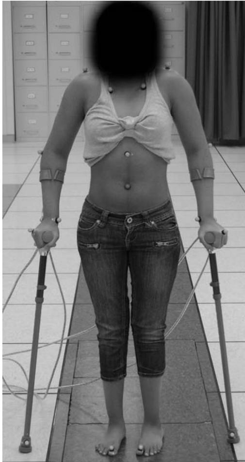
**Figure 1.** Patient with osteogenesis imperfecta (OI) using Lofstrand crutches. She is instrumented with the UE marker system and is using the kinetic Lofstrand crutches.
