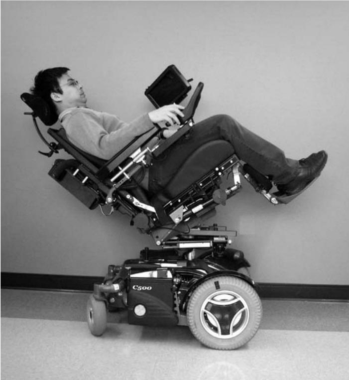
**Figure 5.** Investigator using the wheelchair instrumented with Virtual Seating Coach. The Virtual Seating Coach is an instrumented power wheelchair that has multiple sensors to detect and provide real time feedback to wheelchair users to appropriately use power seat functions.
