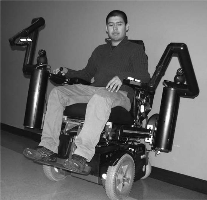
**Figure 4.** Investigator using the PerMMA. PerMMA is a robotic mobility and manipulation device consisting of two coordinated arms to manipulate the objects in a power wheelchair user’s environment allowing individuals with severe disabilities to independently perform activities of daily living.
